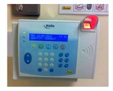
the Internet to the Solihull HQ. Each employee simply touches the screen and the scanner captures the fingerprint which is compared against a stored profile to identify the employee. This is then transmitted to the central control software which then provides real time data reports tailored for specific departments.
