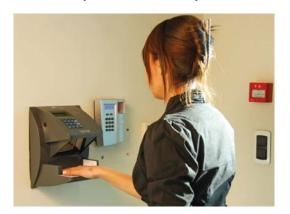
off. Staff members simply place their hand onto the scanner which captures a handprint. This is then fed directly to the software on the central server which compares the handprint against a stored profile to identify the employee and time stamps the record.
