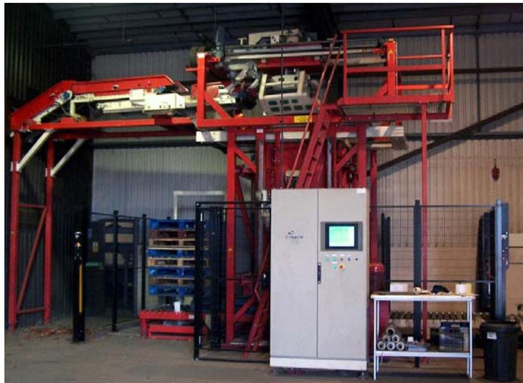
After grading, quality control inspection and automated weighing and filling, the 10kg onion nets were previously stacked onto pallets by hand. This was labour intensive and limited the number of nets that could safely be loaded onto each pallet.
