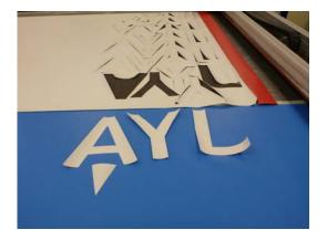
The Genesis automated cutter locks the material in place on a vacuum bed while a computer controlled blade cuts the material to a programmed pattern which calculates the most efficient layout. This minimises any wastage of material and cutting materials at speeds of up to 1500mm/sec dramatically reduces production time.
