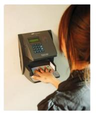
which captures a handprint. This is then fed directly to the software on the central server at the London HQ which compares the handprint against a stored profile to identify the employee and time stamps the record. This not only eliminates our crewhaving to complete time sheets, but the system is also foolproof, providing an accurate real time record of who is on site, when they arrived and when they completed their shift.
