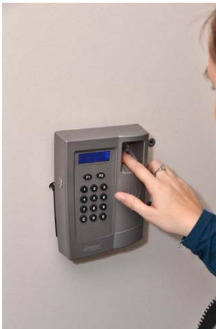
The new system, supplied and installed by Bodet Ltd, streamlines clocking on or off as each staff member simply places their finger onto the biometric reader pad as they arrive or leave. The fingerprint is compared against a stored profile and the identity and time record is sent directly to the Kelio Integral software on the main server which then generates customised reports of time and attendance for payroll and operational management teams.
