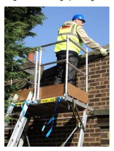
The standard Trim-Line consists of two end platforms, each 1.2 metres long. Each of these can be erected in only 5 minutes and used as independent platforms. Connecting them with the standard 4.6 metre Cat-Walk creates a safe working platform extending to 6.5 metres. The optional 6.6 Cat-Walk increases the working length to 8.5 metres. An End Support Frame is also available allowing Trim-Line to be erected in tight boundaries where ground access is restricted to as little as 15 cms.
